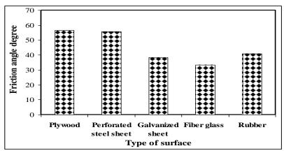
Fig. (8): Friction angle for raw material on different surfaces.
