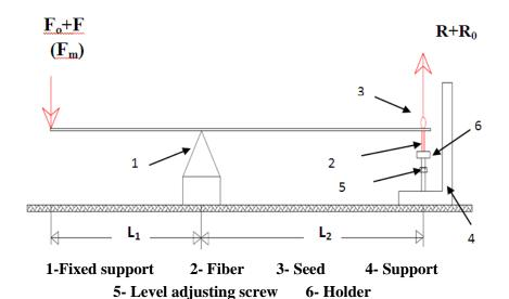
Fig. (5): Lever setup used for amplifying the force measured by the digital force gauge.
