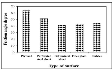
Fig. (7): Friction angle for fibers on different surfaces.
