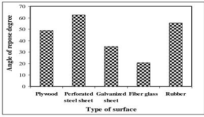
Fig. (9): Angle of repose for seeds on different surfaces.
