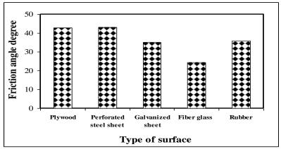
Fig.(6): Friction angle for seeds on different surfaces.
