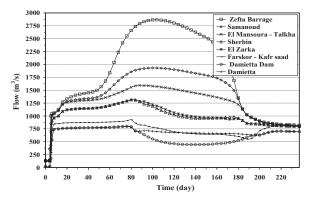
Figure (5): Hydrographs at different sites cross 2<sup>nd</sup> and 3<sup>rd</sup> reaches of Damietta Branch
