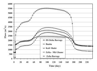
Figure (4): Hydrographs at different sites across 1<sup>st</sup> reach of Damietta Branch
