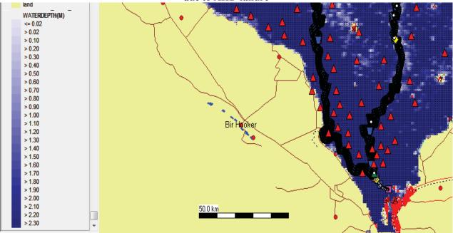
Figure (19): GIS map of inundated areas of Delta Lands after 4 months due to AHD failure
