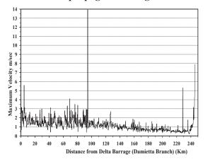
Figure (9): Max. velocity along Damietta Branch
