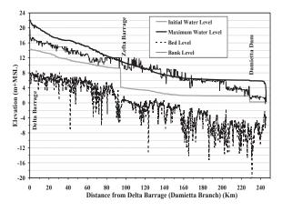
Figure (16): Peak water profile on Damietta Branch
