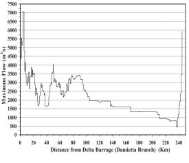
Figure (10): Max. flow along Damietta Branch
