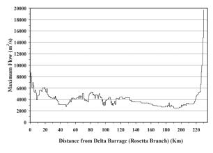
Figure (15): Max. Flow along Rosetta Branch
