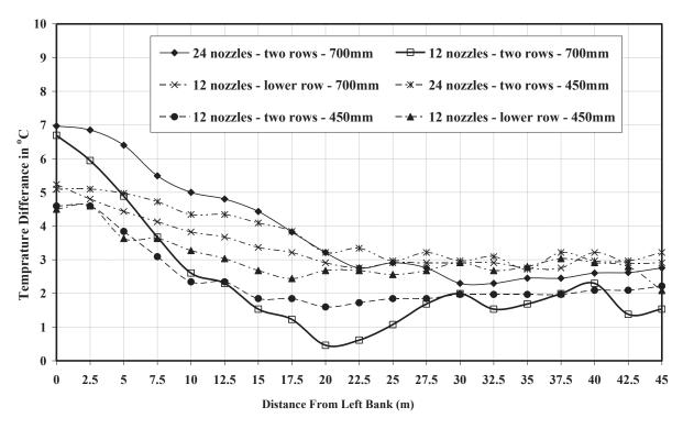
Figure (6): Thermal cross section at 85 m downstream of the outfall axis
