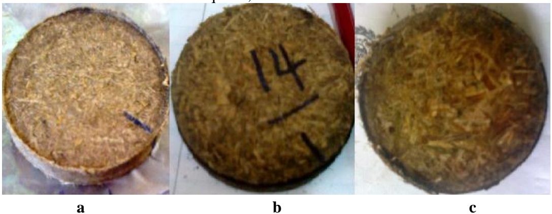
Fig. (3): Specimens of rice straw briquettes (a: without heat, b and c are heated at 75 °C and 100 °C, respectively) after pressing and before testing.
