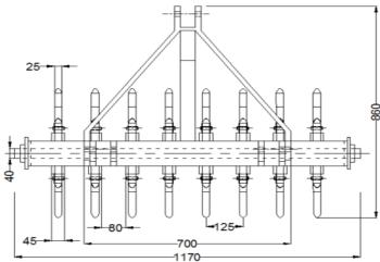
Fig. (1): Elevation of aeration machine.
