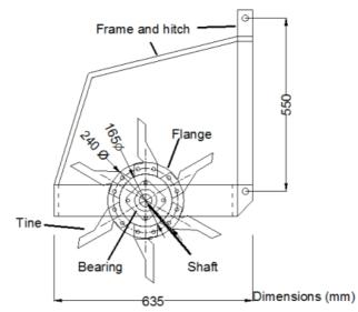
Fig. (2): Side view of aeration machine.
