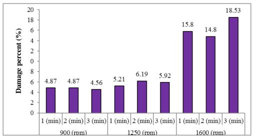
Figure (5) Effect of the machine velocity and operating period on damage percent for type of olive (*Krotina*) without spraying.
