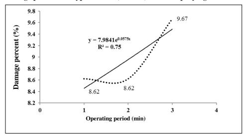
Fig. (6) The relationship between the operating period and harvest damage percent for olive type (Krotina) without spraying.
