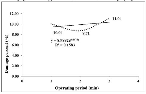
Fig. (10) The relationship between the operating period and harvest damage percent for olive type (*Manzanilo*) without spraying.
