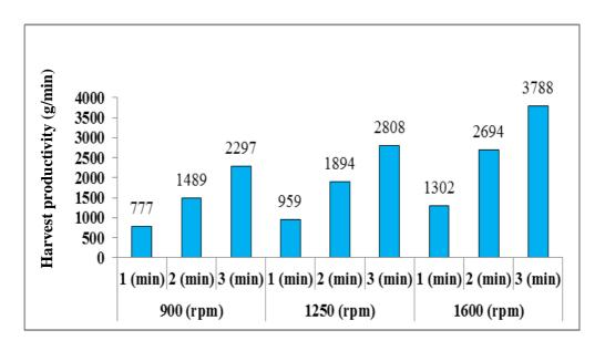
Fig. (11) Effect of the machine velocity and operating period on harvest productivity for variety of olive (*Kronaky*).
