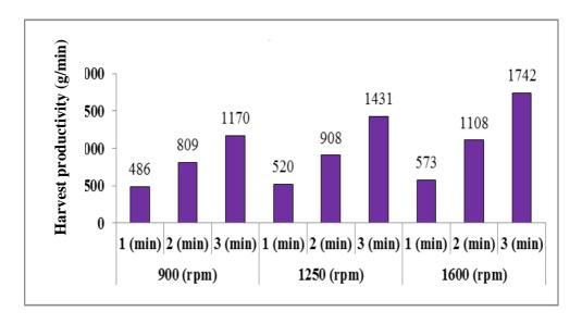
Fig. (3) Effect of the machine velocity and operating period on harvest production for variety of olive (*Krotina*).
