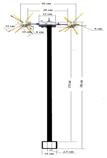
Fig. 1: Front view of hand-held harvester.
