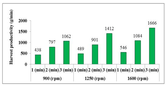
Fig. (7) Effect of the machine velocity and operating period on harvest productivity for variety of olive (*Manzanilo*).
