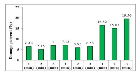
Fig. (9) Effect of the machine velocity and operating period on damage percent for type of olive (*Manzanilo*) without spraying.
