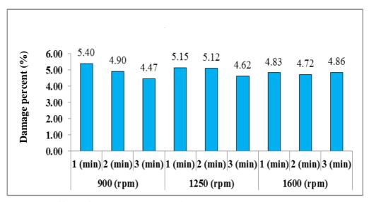
Fig. (13) Effect of the machine velocity and operating period on damage percent for variety of olive (*Kronaky*).
