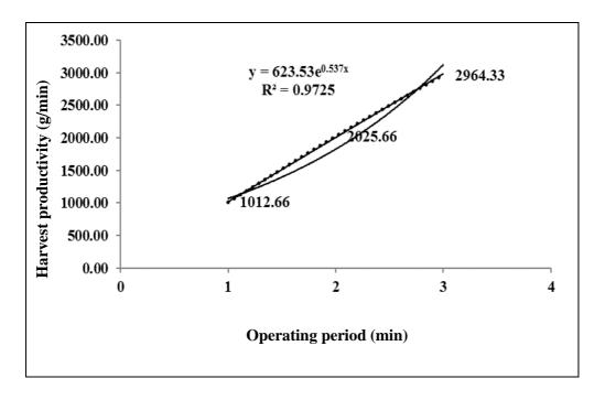
Fig. (12) The relationship between the operating period and harvest production for type of olive (*Kronaky*) without spraying.
