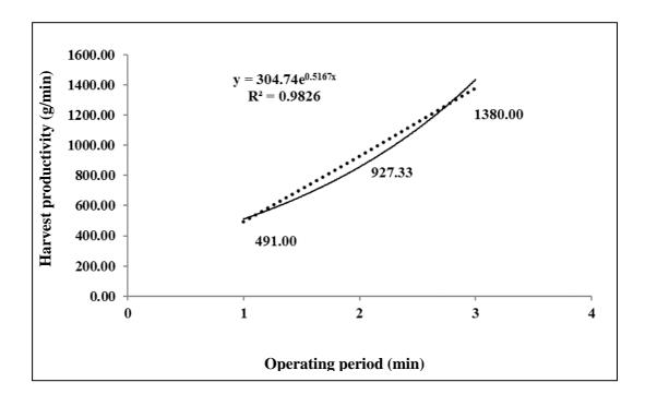
Fig. (8) The relationship between the operating period and harvest production for type of olive ((Manzanilo) without spraying.
