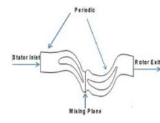
Figure 1: Section of Computational Domain
