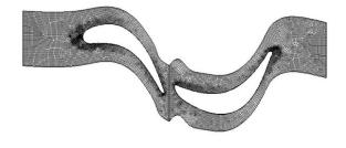
Figure 2: Section of stage mesh
