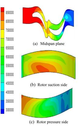
Figure 6: Contour of static pressure (Pa)
