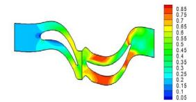
Figure 9: Contour of absolute Mach number at midspan plane
