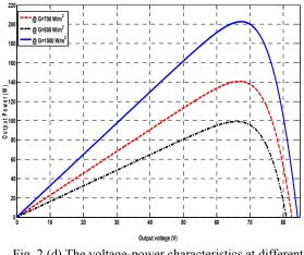
Fig. 2 (d) The voltage-power characteristics at different solar radiation and T = 25c.
