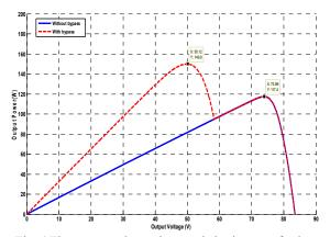
Fig. 4 The power-voltage characteristics in case of using bypass diode
