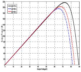
Fig. 2(c)The voltage-power characteristics at different temperatures and  $G = 1000 W/m^2$ .
