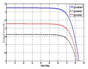
Fig. 2(b) The voltage-current characteristics at different solar radiations and T=25c.
