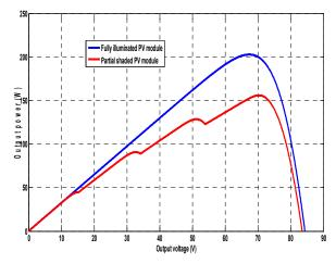
Fig. 3 The voltage-power characteristics in case of fully illuminated and partially shaded PV.
