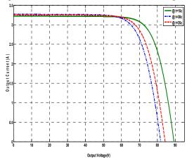
Fig. 2 (a) The voltage-current characteristics at different temperatures and  $G = 1000 \text{W/m}^2$ .
