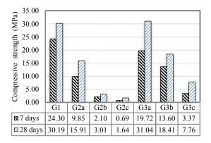
Fig. 5: Unconfined compressive strength of the hardened grouts at 7 and 28 days
