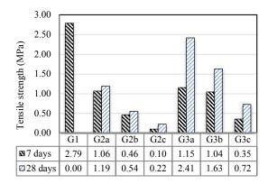
Fig. 6: Indirect tensile strength of the hardened grouts at 7 and 28 days
