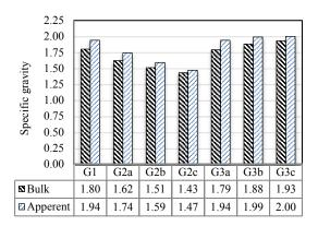
Fig. 4: Specific gravities of the hardened grouts
