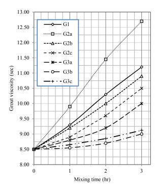
Fig. 3: Effect of mixing time on grout viscosity.
