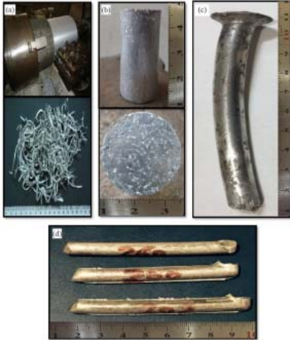
Fig. 1. Solid state recycling stages (a) initial AA-6061 chips (b) cold compacted sample (c) hot extruded sample (d) ECAPed samples.
