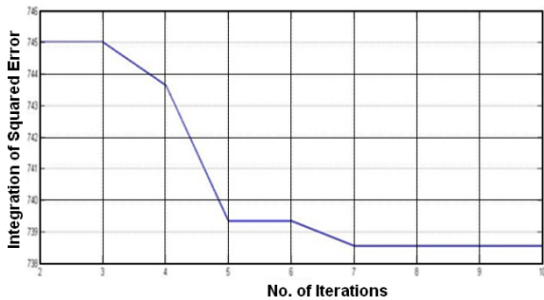
Fig. 8 The objective function versus the number of iterations when using (ALO) for average current control method
