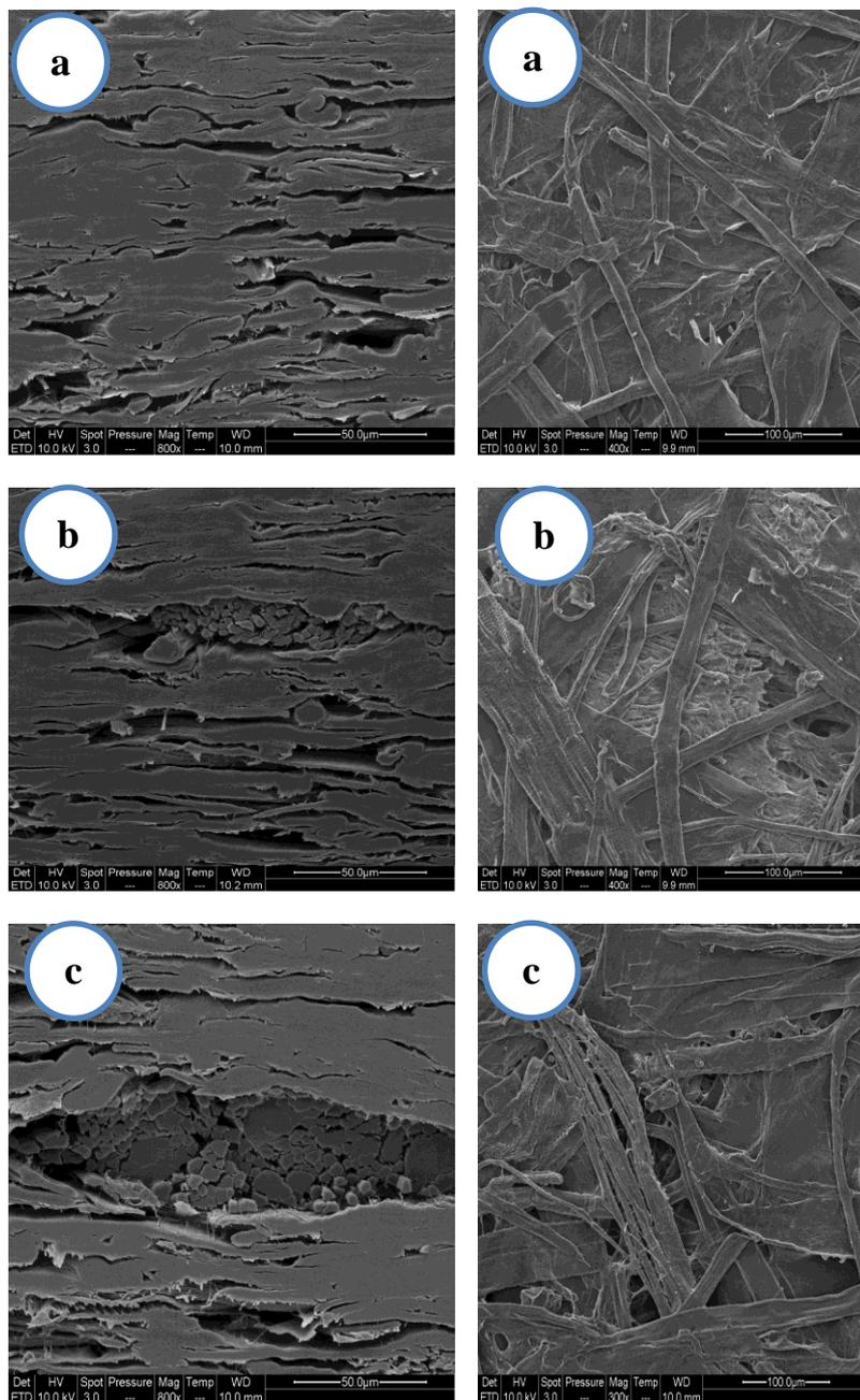
**Fig. 1a.** SEM images of a) blank carton sheet with fracture and surface image as well as carton sheet with different ratios of unmodified leather, b) 6% and c) 12% with fractural and surface image.
