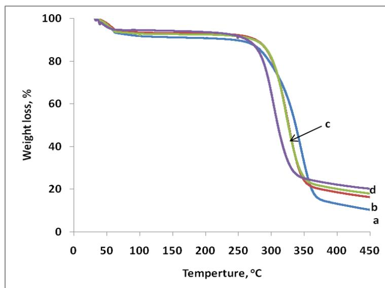
Fig. 2c. TGA of a) blank carton sheet as well as carton sheet with different ratios of treated II, b) 6%, c) 9% and d) 12 %.
