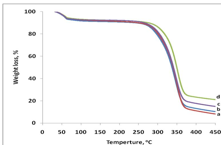
Fig. 2a. TGA of a) blank carton sheet as well as carton sheet with different ratios of unmodified leather, b) 6%, c) 9% and d) 12 %.
