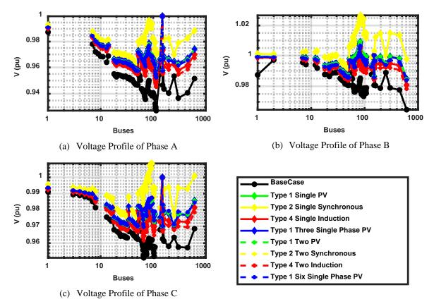
Fig. 8. Voltage Profile of Different DGs of the Three Phases for 123-Bus System by CSA
