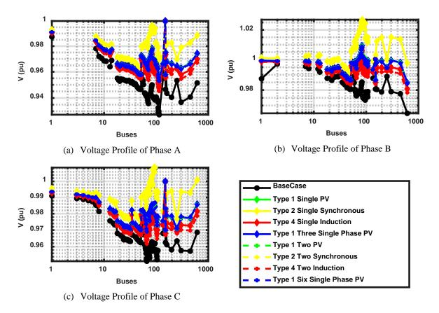
Fig. 9. Voltage Profile of Different DGs of the Three Phases for 123-Bus System by ABC
