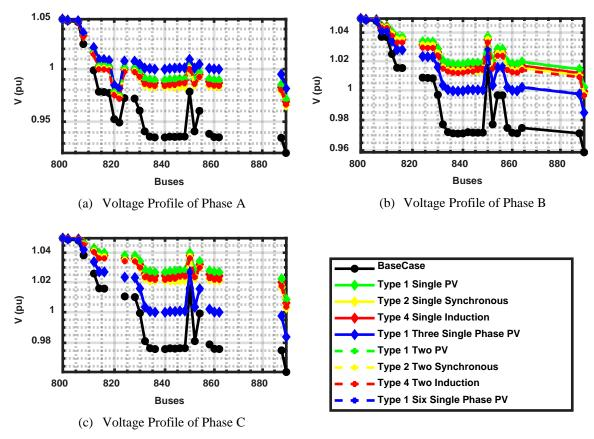
Fig. 7. Voltage Profile of Different DGs of the Three Phases for 34-Bus System by ABC
