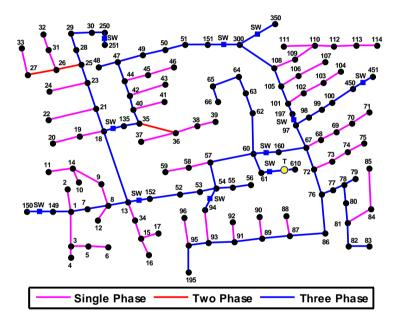
SW: Switch T:Transformer (c) IEEE 123-Bus System Fig. 2.Systems under Study
