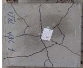
Fig. 22. Fracture mode of 25% FRAC under flexural load.
