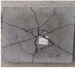
Fig. 17. Fracture mode of NC under flexural load.
