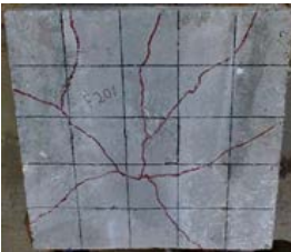
Fig. 21. Fracture mode of 20% FRAC under flexural load.
