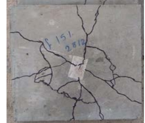
Fig. 20. Fracture mode of 15% FRAC under flexural load.
