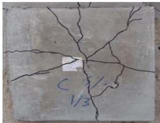
Fig. 25. Fracture mode of 5% CRAC under flexural load.
