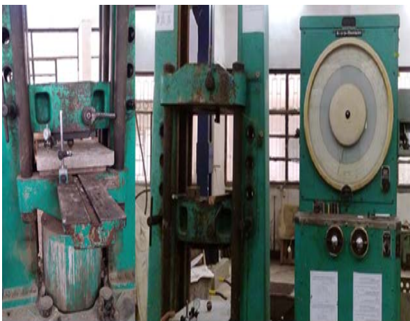
Fig. 2. Set-up of the flexural tests.
