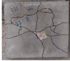
Fig. 18. Fracture mode of 5% FRAC under flexural load.
