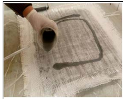
Fig. 2. Spread the micro/nanophased epoxy on the glass fiber layers
