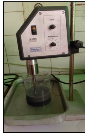
Fig. 1. Mixing Al particles with Ultrasonic processor
