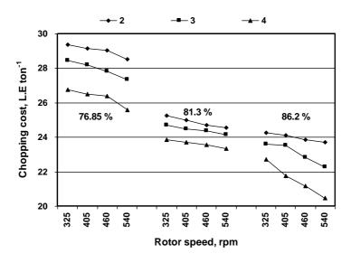
Fig. (13): The effect of moisture content, number of knives rows and rotor speed on the chopping cost.
