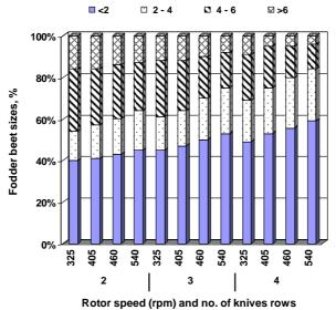
Fig. (8): The effect of number of knives rows and rotor speed on the beet size at 76.85 % moisture content.
