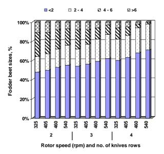
Fig. (9): The effect of number of knives rows and rotor speed on the beet size at 81. 3 % moisture content.
