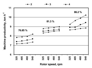
Fig. (11): The effect of moisture content, number of knives rows and rotor speed on the machine productivity.
