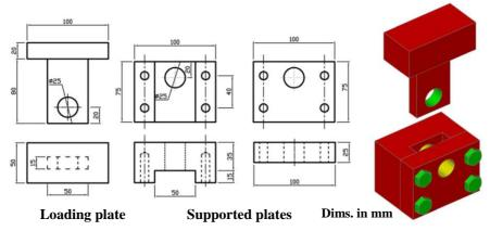
Fig. (3): The shear force measuring device.
