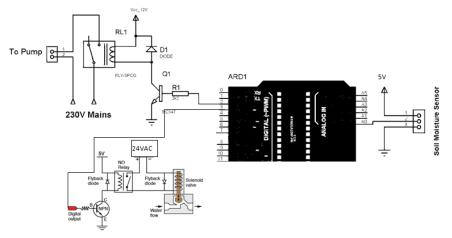
Figure 3. Electric circle of experimental system
