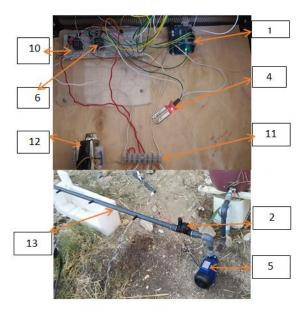
Figure 1: Main hardware of experimental prototype
