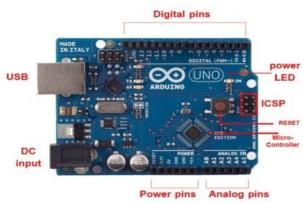
Figure2. Components of arduino board
