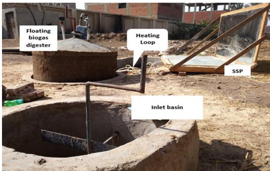
Fig. (1): The Experimental solar-heated biogas digester.
