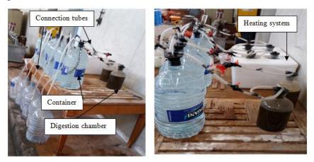
Fig. (1): Biogas digesters parts.
