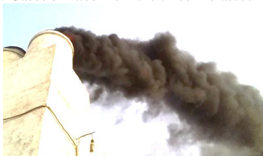
Fig. (6): Smoke intensity from the chimney of factory (c) use bagasse & rubber.
