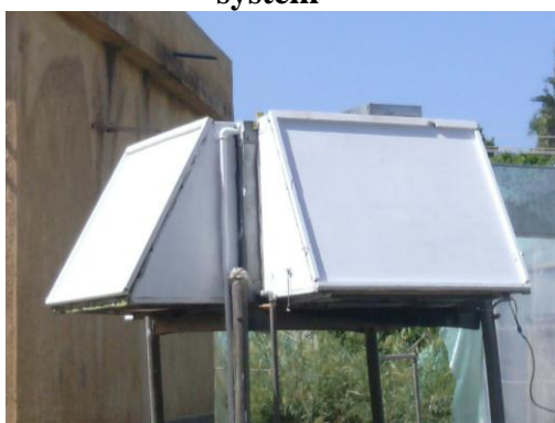
c- Modified evaporative cooling system with desiccant filter housings
