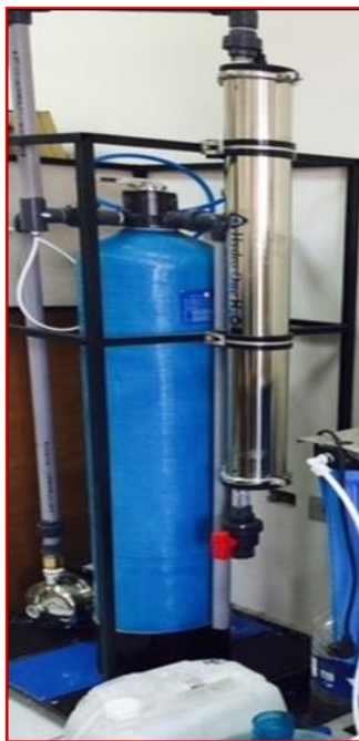
Fig. 3. Installed UF pilot testing machine
