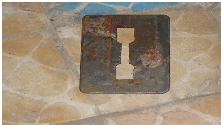
Fig. (2) A special stamp used to control the thickness of adhesive
