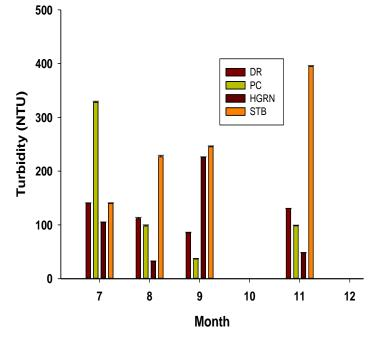
Figure (2): Turbidity of wastewater at four different sites in N'Djamena. Table 5: Heavy metals concentration (mg/l) wastewater of Diguel Ryad (DR)
