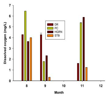
Figure (1): Dissolved oxygen of wastewater at four different sites in N'Djamena
