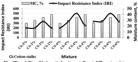
Fig. 8Durability of briquetted cotton stalks at different moisture content with different bending material percentages
