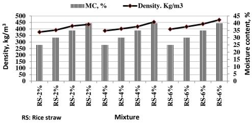
Fig.13 Densities of produced rice straw briquettes at different moisture content with different bending material percentages
