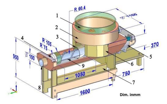
Fig.1 Briquetting machine and its components 1) Hopper 2) Cutting, crushing unit 3) Pressing and extrusion system 4) Die cylinder 5)
