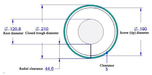
Fig. 4Dimensions of designed extruder screw Table 1: Specification of manufactured screw extruder
