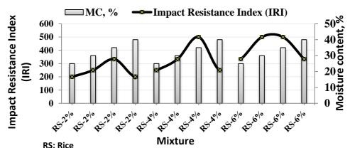
Fig.7Durability of briquetted rice straw at different moisture content with different bending material percentages
