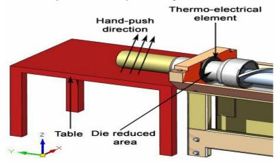
Fig.6Mechanism of disconnecting briquettes from die cylinder
