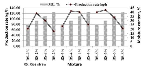
Fig.10 Production rate of briquetted rice strawat different moisture content with different bending material percentages
