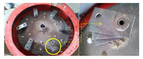
Fig.2 Cutting and crushing unit with blades sets.
