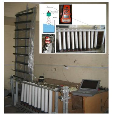
Figure 2: Developmed vertical patternator to measure the vertical uniformity for hydraulic sprayers.
