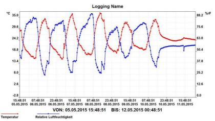
Figure: Measured values of laboratory temperature and relative humidity
