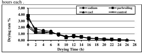
Fig.(4):Drying rate of pretreated tomato slices versus drying time during solar drying.
