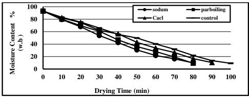
Fig.(5):Moisture content (%) of pretreated tomato slices versus drying time during microwave/hot air drying.
