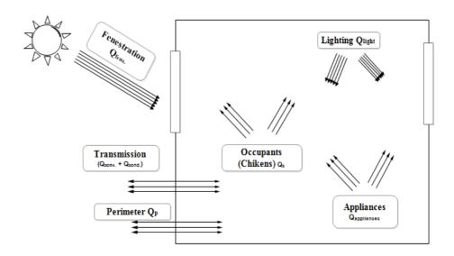
Figure (1): Energy balance of poultry house.
