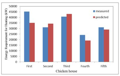
Figure (6): The predicted and the measured energy requirement for heating different poultry houses.
