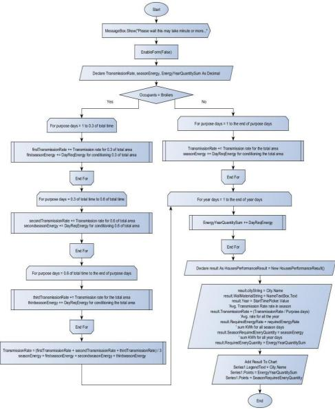
Figure (3): The flowchart of the model.
