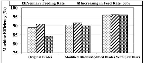
Fig.11. The effect of the blade construction in the machine efficiency
