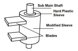
Fig. 4. The modified blade with hard plastic sleeves
