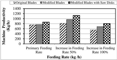
Fig. 10. The effect of the blade construction in the machine productivity
