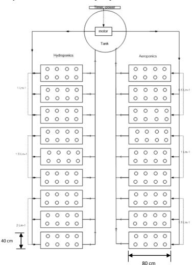
Fig. 1. The experimental setup
