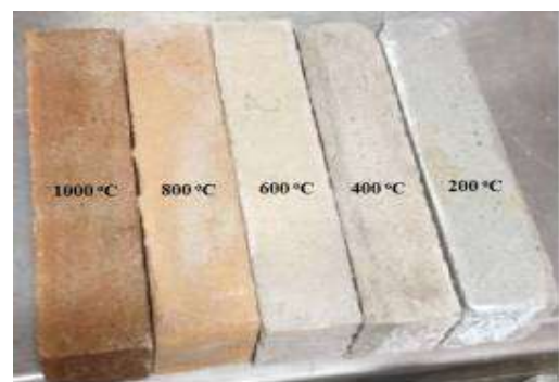
Fig. 19: The effects of elevated temperatures on colour changes of GP mortar specimens
