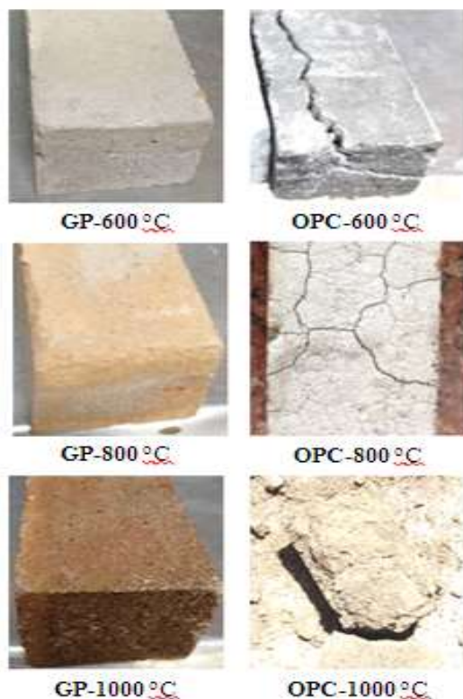
Fig. 20: Damage pattern of GP and OPC mortar mixes as affected by higher temperatures
