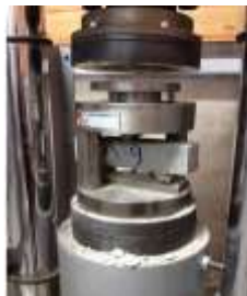
Fig. 3: Flexural test setup
