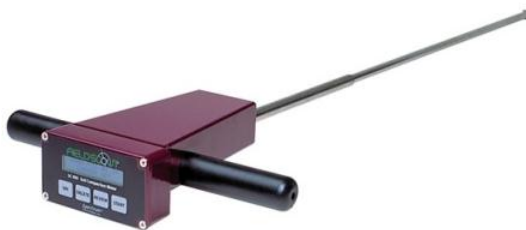
Figure (3). Hand digital penetrometer for measuring soil cone index.
