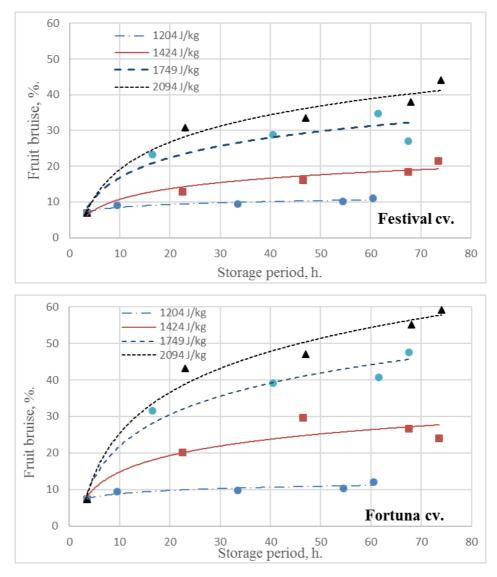
Fig. 6: Effect of storage period after the vibration treatment on the fruit bruise at different energy spectral densities.
