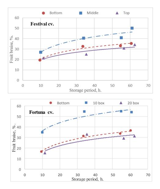
Fig. 7: Effect of storage period after the vibration treatment on the fruit bruise at different box positions on vibrational table.
