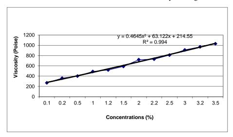
Fig. (1): Relation between concentrations of polyvinyl acetate and viscosities.
