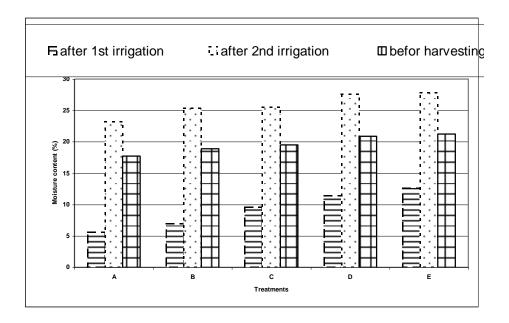
Fig. (2): Effect of polyvinyl acetate concentrations on soil moisture content of the depth (0–5 cm) using the working pressure of 50 kPa.
