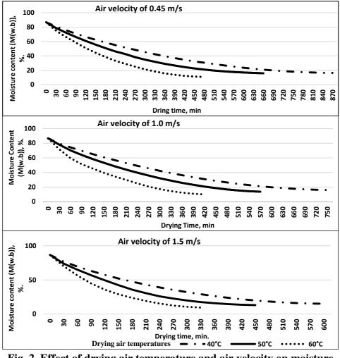
Fig. 2. Effect of drying air temperature and air velocity on moisture content for moringa leaves
