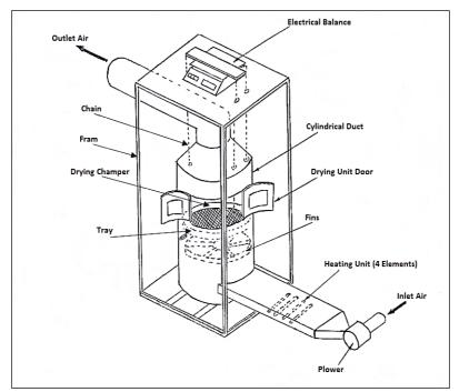
Fig. (1): Schematic diagram of the experimental dryer. <u>Instrumentation:</u>
