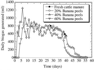
Fig. (4): Daily biogas production of different mixing banana peels with fresh cattle manure
