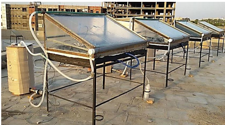
Fig. (1): A photo of the four solar stills with cooling arrangement for glass cover.
