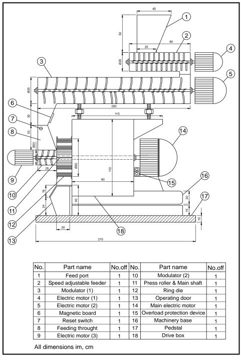
Fig. (1): The schematic drawing of the ring die animal feed pellets extruder.
