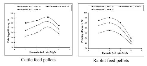
Fig. (4): Effect of formula feed rate and formula moisture content on pelleting efficiency under different kinds of animal feed pellets
