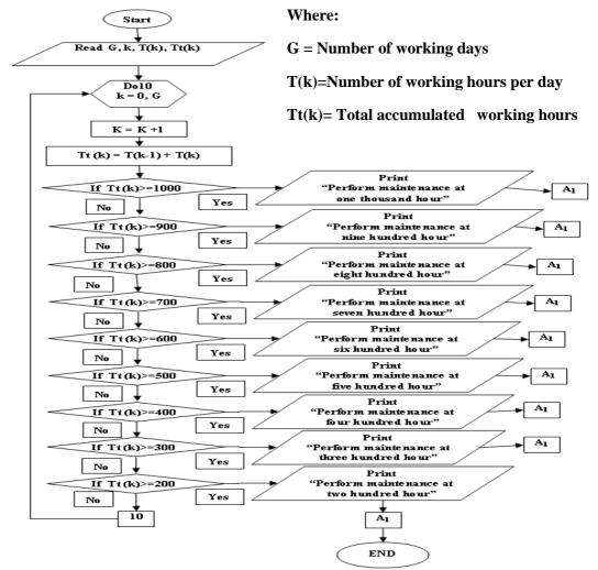
Fig. (10): Program flowchart to determine regular maintenance for farm machinery.
