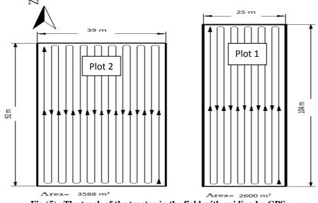
Fig.(5). The track of the tractor in the field with guiding by GPS.
