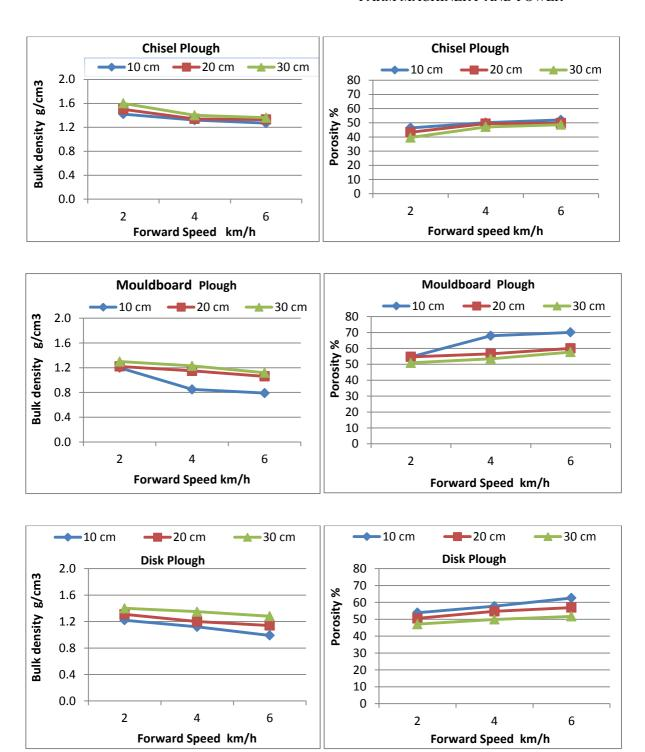
Fig (1): Effect of tillage system on physical properties of soil
