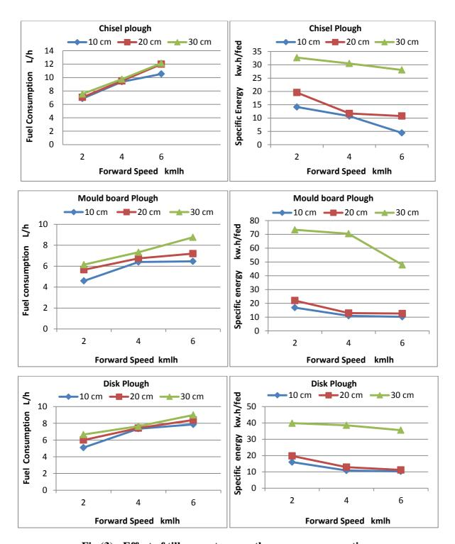
Fig (3): Effect of tillage systems on the energy consumption.
