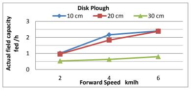
Fig (2): Effect of tillage systems on the field capacity
