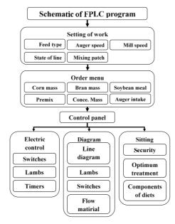
Fig. (7) shows the schematic of the local feed production line control system.
