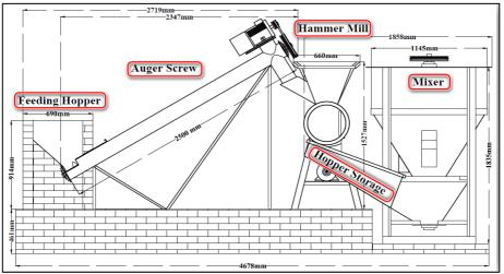
Fig. (2) : The local feed production line.
