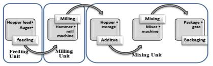
Fig. (1) : The processing stages and units of a local feed production line machine.
