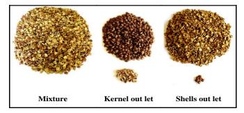
Fig. (7): Result of separation process.
