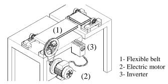
Fig. (5): Feeding rate measurement apparatus.
