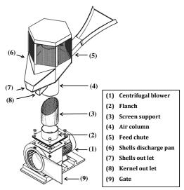
Fig. (3): Assembling of separation unit.
