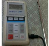
Fig. 4. Air velocity meter and its probe.
