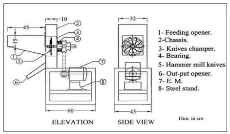
Fig. (1): local hammer mill machine.
