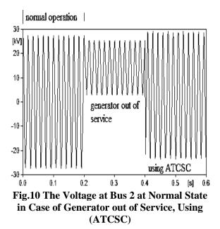
Fig. 11 shows the voltage at bus 2 at normal state from 0 to 0.2 sec. and when generator connected to bus 2 is out of service from 0.2 to 0.4 sec. and when connected Advanced Thyristor Controlled Series Reactor (ATCSR) at bus 2 from 0.4 to 0.6 sec. and the voltage increased to the normal state (voltage=27.3 Kv).
