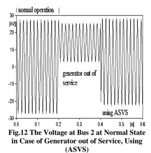
Fig.13 shows the voltage at bus 2 at normal state from 0 to 0.2 sec. and when generator connected to bus 2 is out of service from 0.2 to 0.4 sec. and when connected Advanced Static VAR Compensator (ASVC) at bus 2 from 0.4 to 0.6 sec. and the voltage increased (voltage=27.30 Kv).
