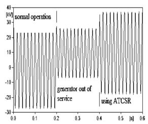
Fig.7 The Voltage at Bus 3 at Normal State in Case of Generator out of service, Using (ATCSR)
