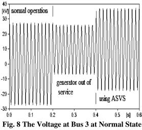
in Case of Generator out of Service, Using (ASVS)
