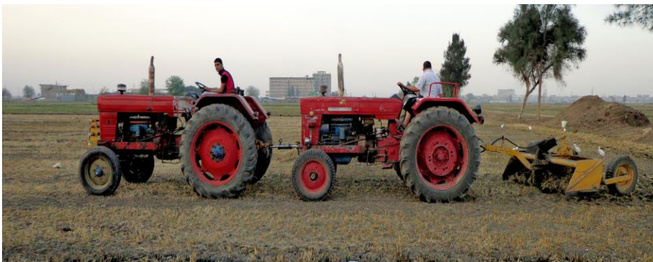
Fig. (2): Pulling force measurement
