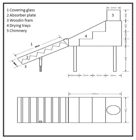
Fig. (1): Schematic diagram of solar drier
