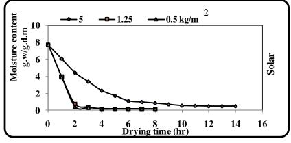
Fig. (5) Moisture degradation during solar drying.
