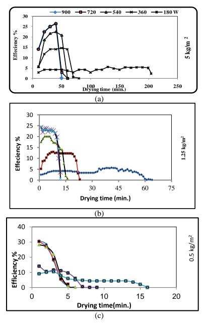
Fig. (8) relation shape between the drying efficiency (%) and microwave drying time(min)
