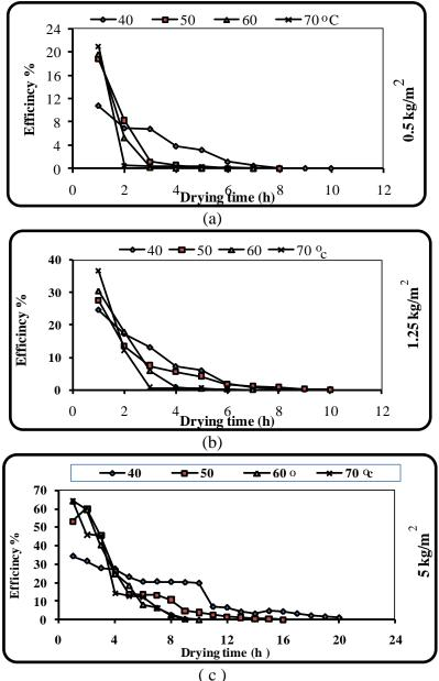
Fig. (6) relation shape between the drying efficiency and oven drying time
