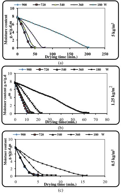
Fig. (3) Moisture degradation during microwave drying.
