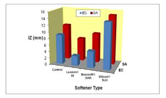
[softener], 20 g/L; pH, 5; wet pick up, 100%; drying, 85  $^{\circ}$ C /5 min; curing, 130  $^{\circ}$ C/3min. Control, linen sample treated with TC in absence of any of softeners. SA: *S. aureus*; EC: *E. coli*.
