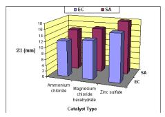
[TC], 10 g/L; [DMDHEU], 50 g/L; [catalyst], 5 g/L; wet pick up, 100%; drying, 85 °C/5 min; curing, 160 °C/3 min. SA: *S. aureus*; EC: *E. coli*.
