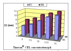
pH, 5; wet pick up, 100%; drying, 85  $^{\circ}$ C /5 min; curing, 120  $^{\circ}$ C /3 min. SA: *S. aureus*; EC: *E. coli.*
