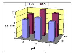
[TC], 10 g/L; wet pick up, 100%; drying, 85 °C/5 min; curing, 120 °C/3 min. SA: *S. aureus*; EC: *E. coli.*
