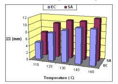
[TC], 10 g/L; pH, 5; wet pick up, 100%; drying, 85 °C/5 min; curing time, 3 min. SA: *S. aureus*; EC: *E. coli.*
