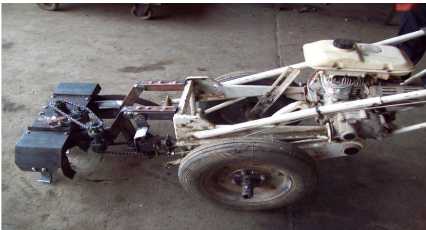
Figure 4: Assembling of power weeder in the workshop and testing the mechanism of motion.
