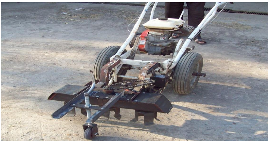
Figure 6: Arrangement done to control the depth of operation during usage of weeder as inter-row method.
