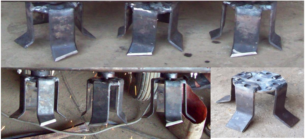
Figure 2: The manufactured modified L-shape blades type with cutting edge.
