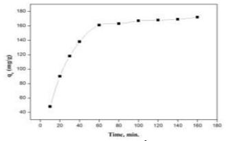
Fig. 3. Effect of contact time on the adsorption of Cu<sup>2+</sup>ions on CMC-g-PAA hydrogel (initial concentration 100 mg/L; CMC-g-AA 0.5 g/L; pH 5; shaking rate 150 rpm).
