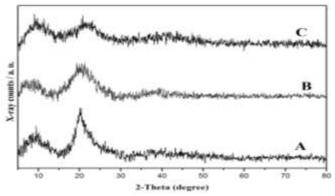
Fig. 6. XRD patterns of (A), CMC (B), CMC-g-PAA hydrogel and (C), copper adsorbed CMC-g-PAA hydrogel samples.
