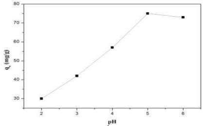
Fig. 2. Effect of pH on the adsorption of Cu<sup>2+</sup> ions on CMC -g-PAA hydrogel (initial concentration 100 mg/L; CMC-g-AA 0.5 g/L; contact time 120 min; shaking rate 150 rpm).
