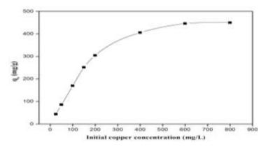
Fig. 4. Adsorption isotherm of Cu<sup>2+</sup> by CMC -g-PAA hydrogel at various initial Cu<sup>+2</sup> concentrations (initial concentration 25–800 mg/L, CMC-g-PAA 0.5 g/L, pH 5, shaking rate 150 rpm).
