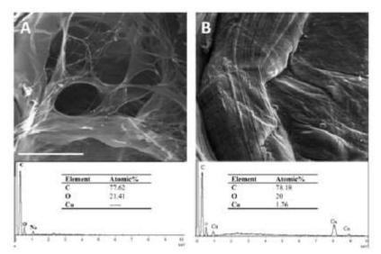
Fig. 7. SEM micrographs and corresponding representative EDX patterns of CMCg-PAA hydrogel (A), before and (B), after the adsorption process in  $Cu^{2+}$  ions solutions( Scale bar =200µm).
