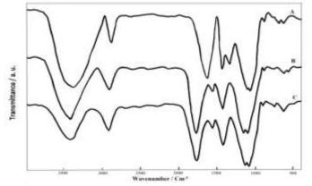
Fig. 5. FT-IR spectra of (A), CMC and CMC-g-PAA hydrogel (B), before and (C), after Cu<sup>2+</sup> adsorption.
